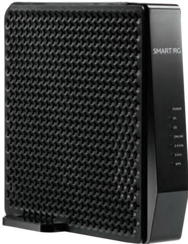
The SmartRG<sup>®</sup> SR808ac is an advanced DOCSIS<sup>®</sup> 3.0 Wireless Cable Gateway, incorporating 24x8 Channel bonding, a 4-port Gigabit Router, High-Power 802.11ac wireless networking -- all built into a single device capable of supporting both residential and small office applications.
