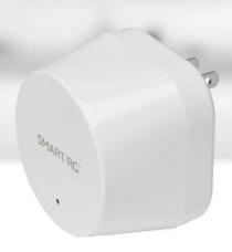
The SE80ac wall plug satellites/access points work with your existing equipment to form an Intellifi® mesh network. Your gateway acts as the hub (controller) and the SE80s act as satellites.
